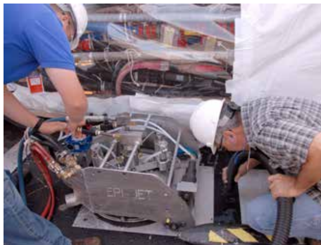
Pearl Harbor Naval Shipyard engineers examine nonskid removal device during course of nonskid material removal trials.
