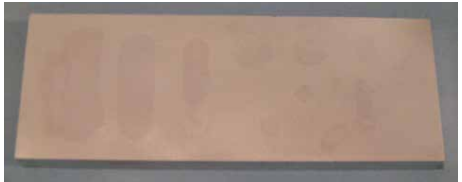
Figure 8. Photograph of the repaired and machined test plate inspected with dye penetrant.
