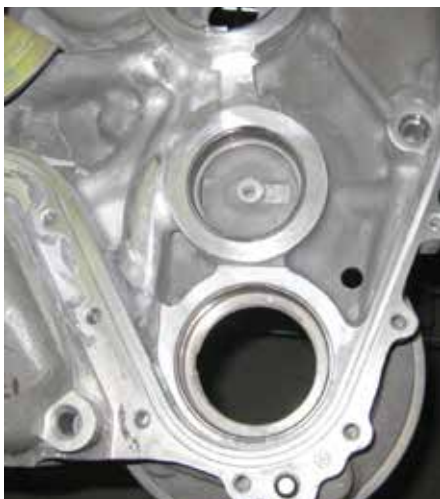
Figure 3. Photograph of repaired AMAD housing which had internal damage.
