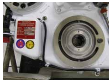
Figure 6. Photograph of the cold spray repaired hydraulic pad.
