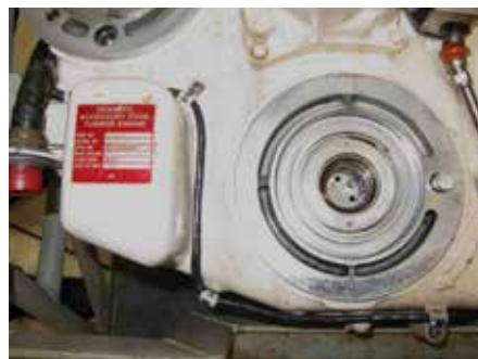
Figure 4. Photograph of a damaged hydraulic pad.
