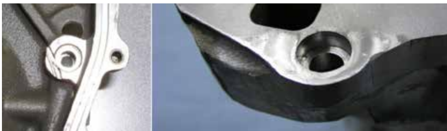
Figure 2. a) photograph of the damaged oil port b) the cold spray repaired oil port on a sub-scale test article.
